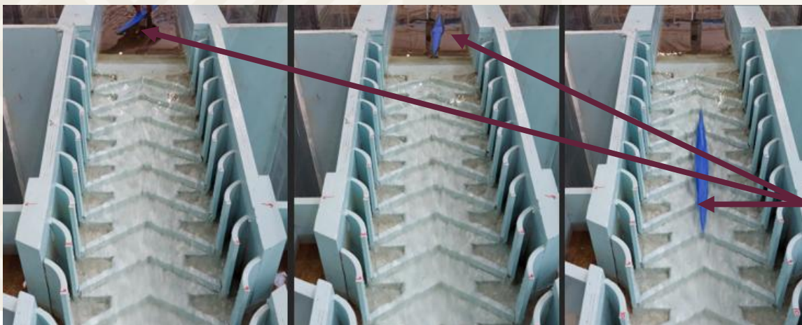
Straightening of angled canoe at entry
