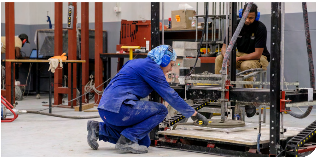
In the 3D-printing laboratory, Dr Kim Timm uses a gantry-type 3D printer to print substantial concrete elements.
