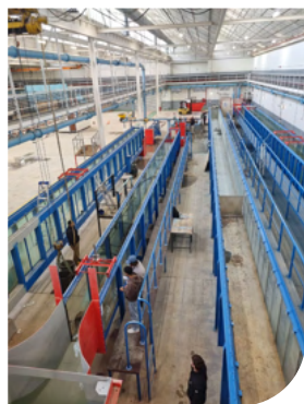
Third-year Hydraulics 354 students turn up for the practical investigation of flow behaviour in an open channel flume. To recommend suitable lining materials for the refurbishment of wastewater canals, they'll use gravel and smooth-bed conditions to determine hydraulic roughness.
