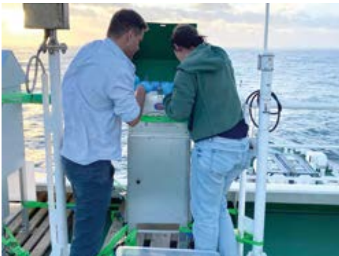
▲ Earth Sciences Postdocs Dr Heleen Vos (right) and Dr Ole Valk (left) changing filters on the high-volume dust sampler over the Southern Ocean during the 2024/2025 Antarctic Relief voyage on board RV SA Agulhas II. Photo: Heleen Vos
